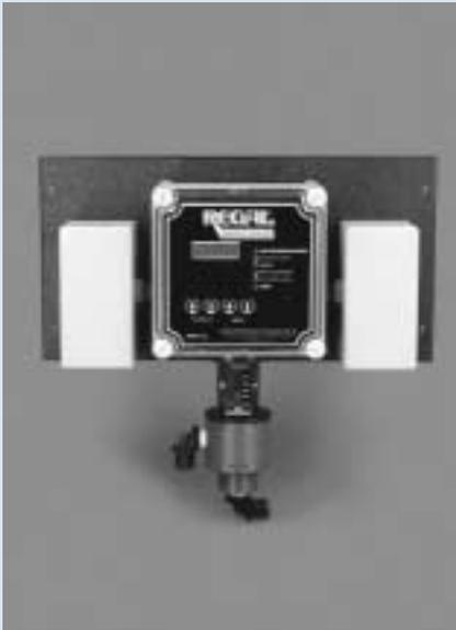
The REGAL SMARTVALVE™ is used for treating water with varying flow rates. Factory-configurable for "flow-proportional" or "step-rate" control mode. Fully automatic or manual operation. Adjustable "low-flow" alarm. Displays flow rate, valve flow position in Pounds Per Day of actual gas feed rate; mode of operation and dosage value. Microcontroller keeps valve linear when dosage is set at 1:1. Chlorine service to 2000 PPD. Sulfur dioxide service to 500 PPD.
