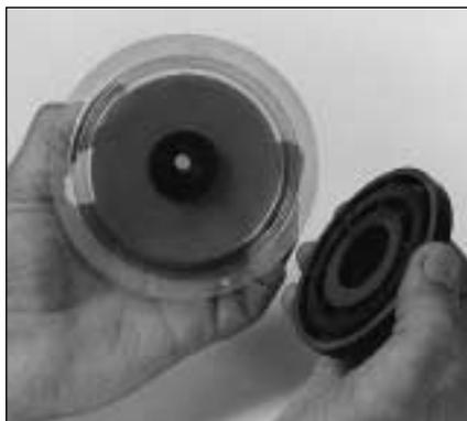
It is the diaphragm which opens the inlet safety valve to allow the gas to flow, and which maintains a steady flow of gas while the system is in operation. Any damage to the diaphragm — even a tiny crack or pinhole — would prevent it from performing these functions. And continuous exposure to the gas would cause these problems if the REGAL diaphragm were not twice as thick and three times as strong as its competition, and made of a plastic that will not corrode.
